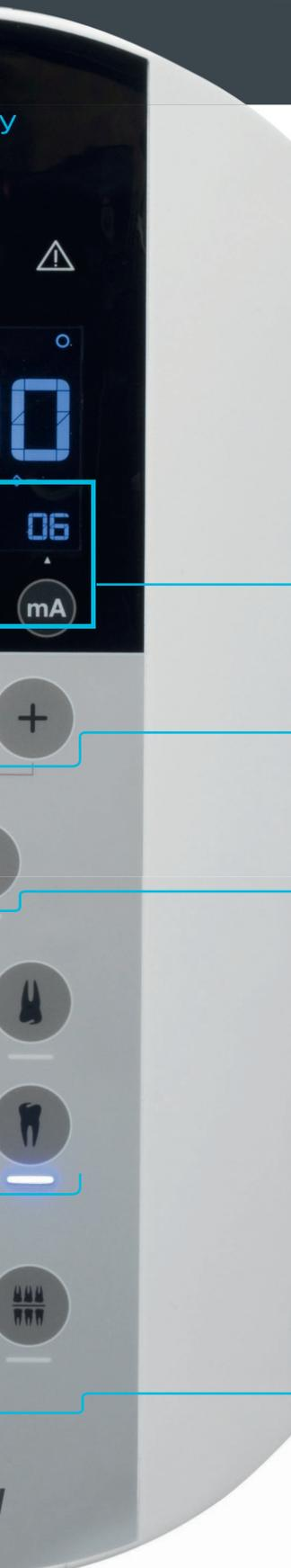
• Displays **THE PARAMETERS** kV, mA, type of film and ACE selection (SOPIX® inside)
